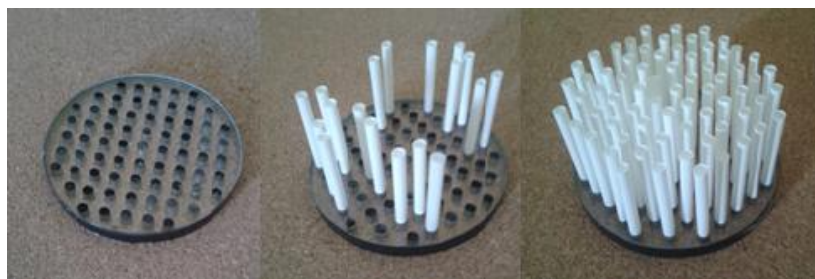
Figure 3. The test samples, from left to right the MPP, MPP attached with eighteen tubes, and the fully attached tubes MPP.
